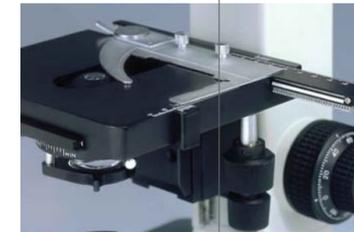
Triangular rail guided mechanical stage balling bearing
