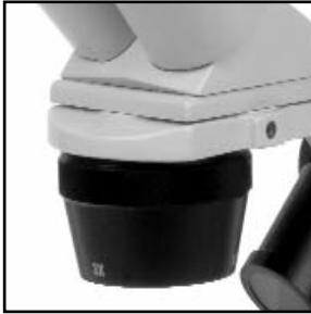
Smooth-moving turret for easy magnification change
